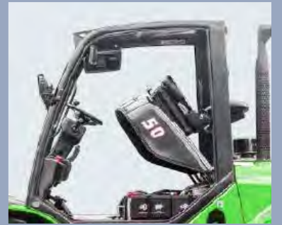
The easy-to-open hook provides quick access to the engine compartment
